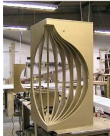
Plywood male and female mould
