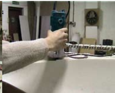
Seam preparation by trimming
